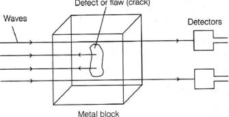
To detect flaws or cracks in metal block, waves are passed through it. If there is even a small defect, the waves get reflected back indicating the presence of the flaw or defect shown in the figure.
